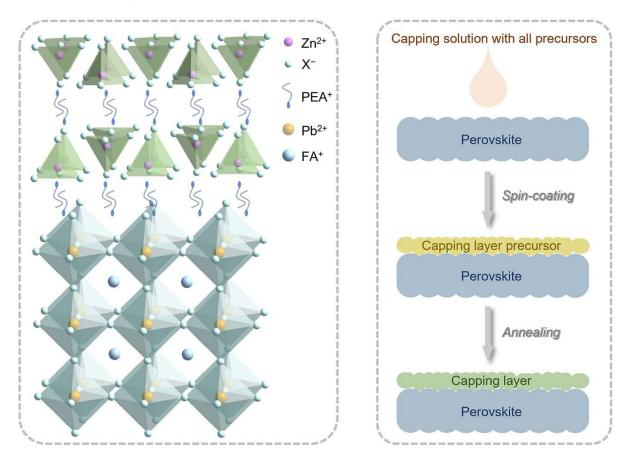
(Left) The molecular structure of perovskite (blue) with the zinc-based capping layer (green). (Right) The FP process that the researchers used to coat the zinc-based capping layer onto the perovskite layer. Credit: NTU Singapore.
